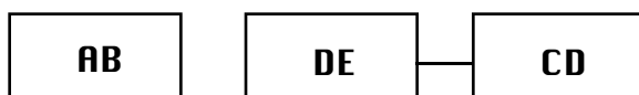
Figure 5a. Junction tree for SM, in and of itself. The cliques are disconnected; information about A or B does not change belief about C, D, or E.
